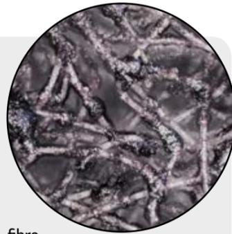
The Klingspor NUD 500 disc is made up of multiple compressed layers of nylon fibre non-woven material. A special application process is used to evenly apply a mixture of silicon abrasive grit and bonding agent on the layers of non-woven material. This procedure ensures that the user can always rely on a fresh, unused abrasive grit, affording them a constant service life.
